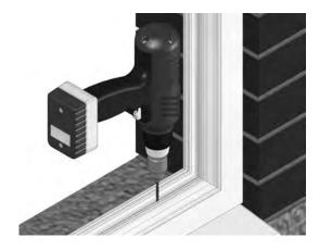
In dwarf wall models use the relevant drill bits to pre-drill two holes through the French door outer frame, as indicated below and then into sound masonry positioned 50mm in from the top and bottom of the dwarf wall.
