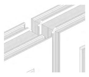
Select the 18mm inline coupling (A104) sliding downwards and through the gap between the two panels until it rests on the 150mm sill (P106) at the foot of the panel.
