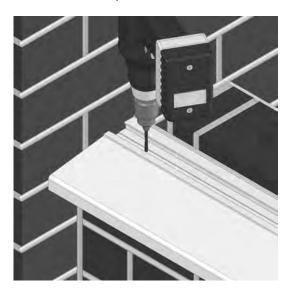
Now permanently fix through the 150mm sill (P106) to the base using the 100mm fixing bolts (PA6).
