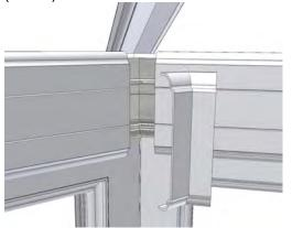
Prior to installing the internal boss cover, it may require trimming to suit the roof pitch.
