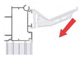
Hang the front edge of the gutter onto the bracket and rotate up the back of the bracket as shown. Fit only to the first "click", do not push all the way up.
