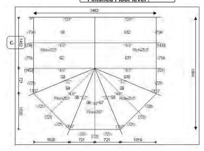
Please note that the end dimensions are taken from the external frame to the centre line of the next rafter. The intermediate dimensions are taken from bar centre line to bar centre line. The image above is an example roof plan. The detail specific to your conservatory is shown on your roof plan, do not follow the dimensions shown in this image.
