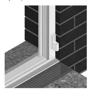
The 18mm inline couplings (A104) are assembled into the gap between the French door outer frame. Remember to silicone seal around the bottom of the 18mm inline coupling (A104) when in position.
