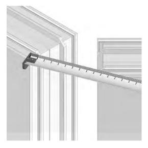
Select the first 135° corner post (A110) and from above, slide between the two adjacent panels. The large angled face section of the 135° corner post (A110) is positioned to the outer corner of the 150mm sill (P106) as shown below. Bed onto a bead of silicone positioned onto the 150mm sill (P106).
