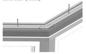
Please note: Do not use the 4.8 x 120mm yellow screws to fix the eaves beam (A5080) to the French door outer frame. Instead use four 70mm fixing screws (70fix) as you used to fix the French door outer frame to the 150mm sill (P106), pre drilling upwards from inside the French door outer frame and up into the eaves beam (A5080).
