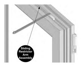
Locate the button on the sliding arm into the receptor of the fixed restrictor assembly. Push firmly upwards until the button snaps into place.
