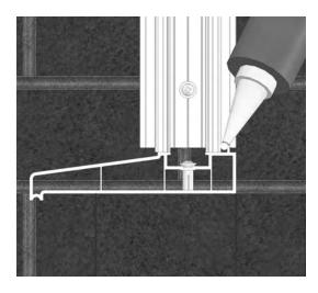
Once level and in the correct position, fix the French door outer frame to the 150mm sill (P106) by use of four 70mm fixing screws (70fix), two positioned on each side of the shoot bolt keeps at the foot of the French door.
