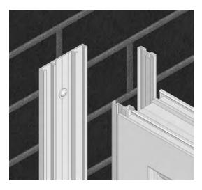
When the two-part connectors are in position, slide the panel towards the 26mm wall connector A105). The leg detail of the two-part connectors (A112) will automatically mate with the leg detail of the forthcoming component.
