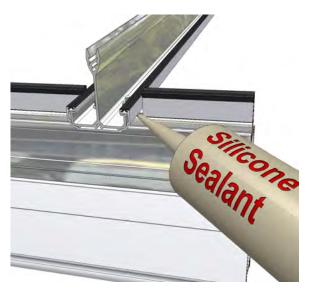
The end closure (P6054) may be preassembled on polycarbonate roof glazing sheets, however you will need to remove the end closure and apply a line of silicone along the top face of the breather tape, the re-fit the end closure. Clean off all excess silicone.
