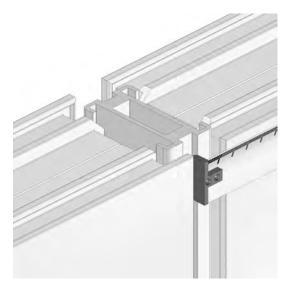
Another application of silicone should be made to the 150mm sill (P106) where the 18mm inline couplings (A104) make contact. This should be a bead 18mm in length and positioned as shown below.
