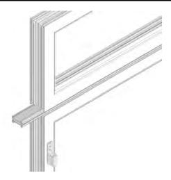
The panels are permanently fixed together in the same way as any other panel using the quarter turn buttons (C105) and the 6mm Allen Key (6AK) as described previously.
