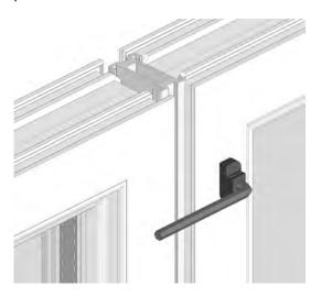
When the quarter turn button (C105) is in position and resting against the 18mm inline coupling (A104), turn the 6mm Allen key (6AK) 90° clockwise. The quarter turn button (C105) will 'click' into position.
