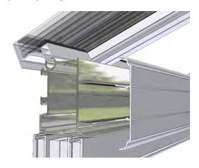
Select the eaves beam 135° cover trim (C9111), and push home into the corner gaps between the eaves beam cover (P6042).
