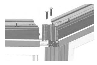
When the eaves beam (A5080) is assembled on top of the panels, drill through the eaves beam (A5080) only with a long reach 5mm drill at positions which are 100mm from the edge of each panel (i.e. two holes per panel position).
