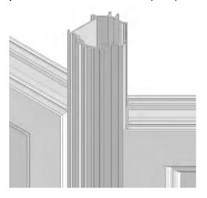
Ensure that the leg detail on the 135° corner post (A110) interlocks with the leg detail on the panels as shown at the top of the next column.
