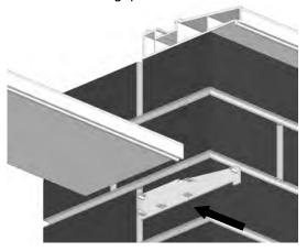
Do not fit the 150mm sill end caps (C101) to the open ends of the 150mm sill either side of the dwarf wall opening until all panels are fitted (with the exception of the French door outer frame which should be positioned last).
