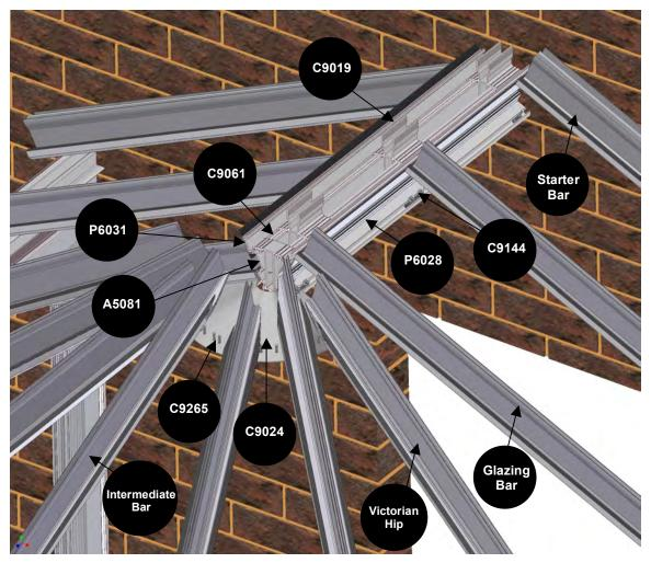
Referring to your roof plan, select the correct number of bolt retainers (C9144) and slide into the channels of the universal ridge wings (A5081).
