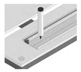
Again, using the scribed vertical line drawn on the wall earlier, position the 26mm wall connector (A105) so that the internal edge is in line with the scribed line on the wall. You will notice that the inside edge of the 26mm wall connector (A105) is in line with the internal face of the 150mm sill (P106). Use a spirit level to check for plumb.
