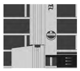
If any marked positions for the 60mm fixing bolts (PD5) land on mortar joints adjust accordingly so that they locate over solid brick. Holding the 26mm wall connector (A105) in position and
