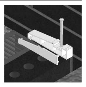
A quick measurement check between the host wall/start position and the 150mm sill end cap (C101) should show 26mm.
