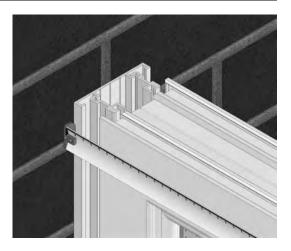
An application of silicone should be made to the 150mm sill (P106) where the two-part connector (A112) has made contact.
