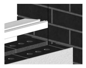
Ensure that every run of 150mm sill (P106) has two 70mm sections on one end of the sill milled out as shown in the image below (with the exception of a cut sill for a French door opening which is described in the next paragraph). This will allow the panels to be slid into the groove of the 150mm sill (P106) throughout installation.
