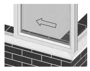
If you have a dwarf wall model conservatory and you have had to cut the 150mm sill (P106) for a French door opening, the first panel, and any subsequent ones between the host wall and the French door opening, are slid on through the open face of the 150mm sill (P106) as shown on the next page.
