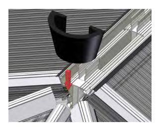
Using the silicone provided, run a continuous bead around the joint between the foam bung (C7023) and the end of each bar top cap, being careful to avoid gaps in the sealant.
