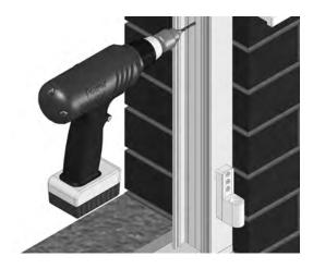
Permanently fix the aluminium low threshold (A103) to the base by use of the 100mm fixing bolts (PA6). The French door outer frame is also permanently fixed to the faces of the dwarf wall by use of the 100mm fixing bolts (PA6).
