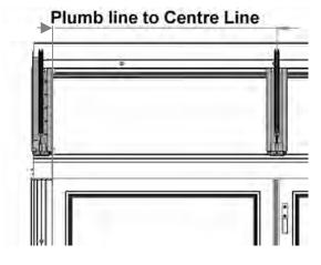
The next dimensional checks are the ones between the intermediate rafters. These dimensions shown on your roof plan are taken from *bar centre line to bar centre line*. If all bars are correctly positioned, tighten the M5 flange nuts.
