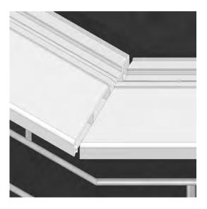
It is recommended that the inside edge of the 150mm sill (P106) is drawn onto the host wall. This guide line will ease in the positioning of the 150mm sill (P106) and the first panels.
