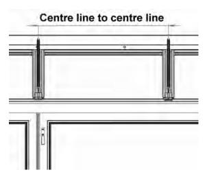
If all checks have been performed it is now possible to permanently fix the starter bars to the host wall.
