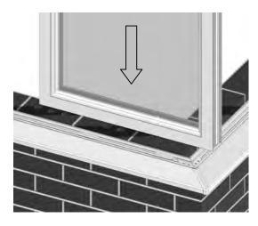
Position the panel onto the 150mm sill (P106) and slide into position.
