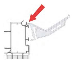
Pull the bracket downwards until it locks into place
