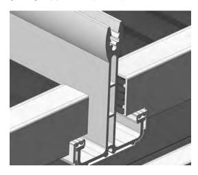
Once the roof glazing sheet is in place, pull on the glazing tape protective film on the glazing support trim (P6056) from the inside of the conservatory in a downwards motion to remove.
