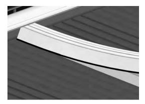
Use a glazing mallet or similar plastic surfaced mallet to knock on the bar top cap starting at the top and working down the bar top cap towards the eaves beam (A5080).
