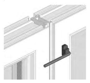
When the quarter turn button (C105) is in position and resting against the 18mm inline coupling (A104), turn the 6mm Allen key (6AK) 90° clockwise. The quarter turn button (C105) will 'click' into position.
