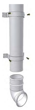
Connect the downpipe shoe (C9013) to the base of the downpipe. Fix the downpipe in position by use of the downpipe retention clips (C8056). They can be clipped over the downpipe and fixed into position with the screws provided
