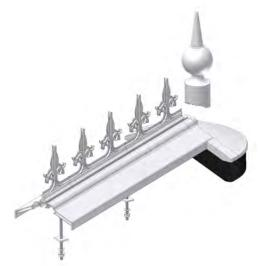
Slide the finial (C7012) fully onto the ridge cap assembly as far as it will go.
