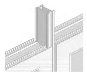
IMPORTANT: As the 18mm inline coupling (A104) is being positioned check that the legs on the 18mm inline coupling (A104) interlock with the leg detail on the panels as shown below.
