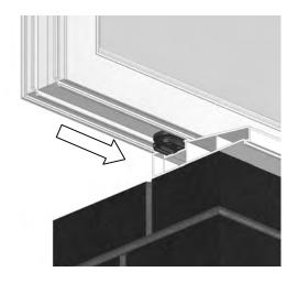
The panel is slid along the 150mm sill (P106) until it is approximately 18mm away from the last panel to be installed.
