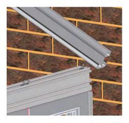
The first check is the distance from the plumb line where you positioned the first panel connector – 25mm connector A (PD4) against the host wall/packing on the far left to the centre line of the next bar (RD6) labelled as 'P2'. Refer to your roof plan for this dimension. If the distance is correct tighten the M5 flange nut fully.
