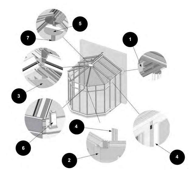
Check that you have sealed the joints in between the glazing support trims and the bar under cladding on each panel and the glazing tape protective film has been removed.
