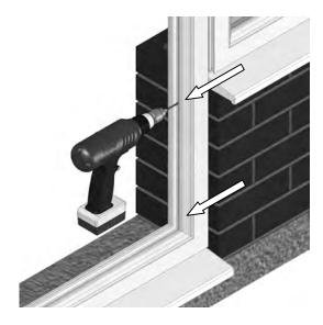
Now permanently fix the French door outer frame to the sides of the dwarf wall with two 100mm fixing bolts (PA6).
