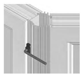
When the quarter turn button (C105) is in position and resting against the 135° corner post (A110), turn the 6mm Allen key 90° clockwise. The quarter turn button (C105) will 'click' into position.
