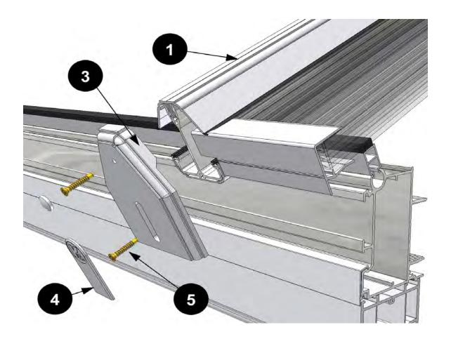
Once all roof glazing sheets are in position and stuck to the glazing support trim (P6056), attach the bar top caps to the bars.
