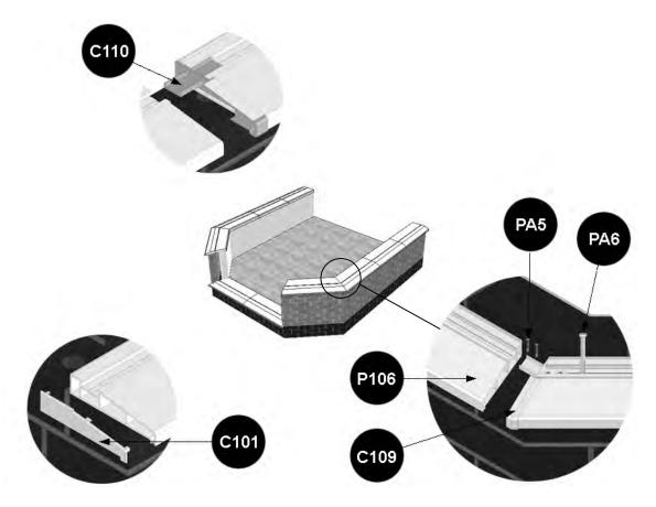
Having already inspected the base for LEVEL AND DIMENSIONAL ACCURACY (against base plan), lay out the 150mm sill pieces (P106) as per the conservatory plan.
