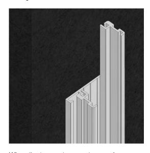
When the two-part connectors are in position, slide the panel towards the 26mm wall connector A105). The leg detail of the two-part connectors (A112) will automatically mate with the leg detail of the forthcoming component. The standard detail is shown on the following page.
