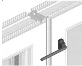
When the quarter turn button (C105) is in position and resting against the 18mm inline coupling (A104), turn the 6mm Allen key (6AK) 90° clockwise. The quarter turn button (C105) will 'click' into position.
