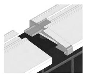
Ensure that the external 135° sill connector (C109) is silicone sealed on all contact areas: top, bottom and sides. Fix all sill connectors (C108/C110) to 150mm sill (PA1) with 3.9 x 16mm reinforcing screws (PA5) as shown below.
