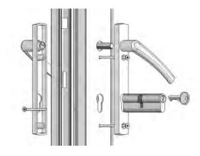
Ensure that the gap between the door sashes is parallel. When set correctly the gap between the doors will be 14mm.
