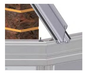
From the underside of the boss end, pass the M5 x 25mm roofing bolts through the pre-drilled holes in the hip and loosely secure with an M5 flange nut.
