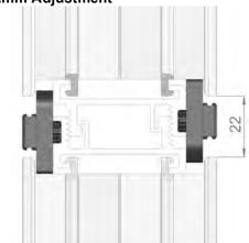
When the adjustable inline couplings (A107) are interlocked to the required setting they are slid between the two adjacent panels in the same way as the 18mm inline couplings (A104).
