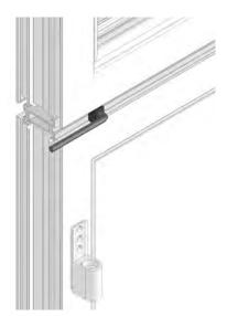
The French door outer frame is positioned like all other panels with the exception that the French door outer frame is not slid onto the 150mm sill (P106) but simply placed into position.
