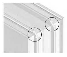
On dwarf wall models, the 18mm inline couplings (A104) which attach the French door outer frame to the adjacent panels are to be cut to size as they must rest on top of the 150mm sill (P106) as shown below.
