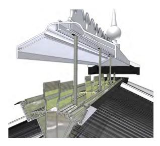
When fitting the external ridge cover assembly, Use of conservatory ladders or boards positioned across the glazing bars will assist spreading any load. Do not put your weight directly on to the roof glazing sheets.
