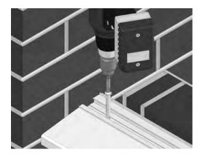
The 100mm fixing bolts (PA6) should be positioned 100mm from each end of the 150mm sill (P106) and equally spaced between.
