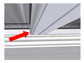
Select the eaves beam cover (P6042), position onto the barbs on the eaves beam (A5080) and press home.
