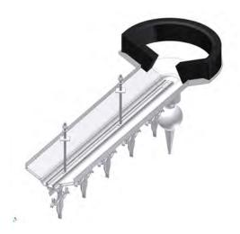
The ridge holding down bolts must be fitted into the groove on the underneath of the external ridge capping at approximately 500mm centres. When fitting the bolts ensure that the nut and washer for each threaded rod is located into the channel, tighten the threaded rod prior to installing.
