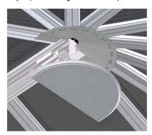
Offer the boss end internal cover (C9028) up to the boss end. The boss end cover internal (C9028) is positioned so that the up stand fits tight against the boss end and the edge against the hip bars.
