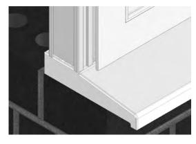
Locate the French door outer frame position by ensuring that the internal face of the French door outer frame is in line with the internal face of the 150mm sill (P106).
