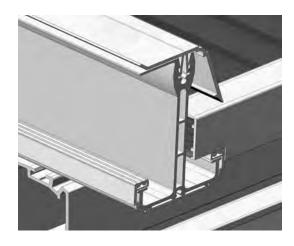
Fix the glazing bar end caps to the end of the bars using two 3.9 x 25mm yellow screws (C8019). Ensure that the top fixing is done first using the cup washer and cover cap, this aligns the end cap bottom holes with the screw port on the glazing bar.
