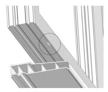
If you have 'TP Panels' these have to be attached to the French door outer frame prior to installation.
