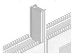
The quarter turn buttons (C105) are positioned longitudinally into the gap between the panels and approximately 50mm from the top and bottom faces of the panel.
