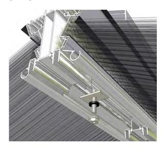
Screw the rectangular washer until it touches the ridge wings and finger tighten the nylon nut on the ridge holding down bolts to make the external ridge capping secure.
