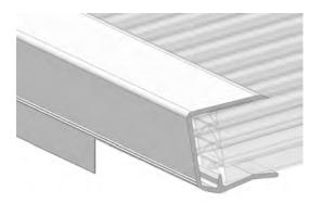
Select the first roof glazing sheet 'G1'and remove its protective films (polycarbonate only). It is recommended that only a 50 to 100mm perimeter of the protective film is removed at this stage as this will help protect the roof glazing sheet from any unwanted marks. The inner protective film can then be completely removed once all plaster work is complete.
