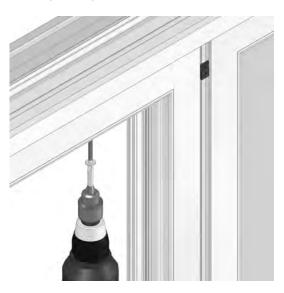
Silicone seal the gaps between the front of the eaves beam external trim (P6024) and the front of the panels to create a water-tight seal.
