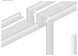
Select the 18mm inline coupling (A104) or adjustable inline coupling (A107) and slide downwards through the gap between the two panels until it rests on the 150mm sill (P106) on the dwarf wall.
