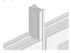
Remember to silicone seal around the bottom of the 18mm inline coupling (A104) when in position.
