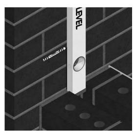
Position the inside face of the 150mm sill (P106) against this line and onto the base.
