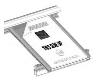
If not already installed, fit all the eaves beam closure (P6056) into eaves beam (A5080). This trim will snap fit into the channels of the eaves beam between the glazing bars. Do not remove the glazing tape protective film at this point.
