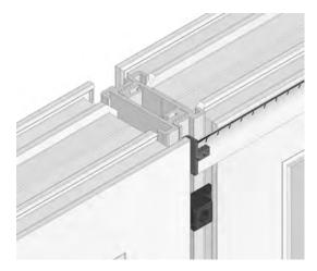
Another application of silicone should be made to the 150mm sill (P106) where the 18mm inline couplings (A104) make contact. This should be a bead 18mm in length and positioned as shown below.
