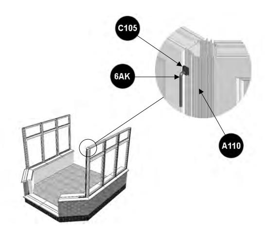
The panels which sit either side of the 135° corner post (A110) should be positioned at the approximate position as shown below so that the external corners of the panels are approximately 75mm apart.
