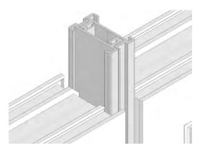
The quarter turn buttons (C105) are again used to lock the panels together in the same positions and quantities as the 18mm inline coupling (A104). A dimensional check is then performed to ensure that the required setting has been achieved.
