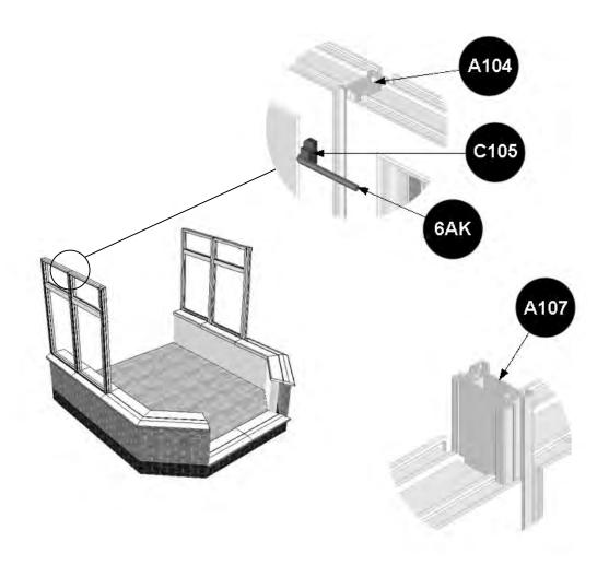
Select the panel to fit against the previously installed panel. It is imperative that the drain slots in every panel are located at the bottom of the panel and facing front as shown below.
