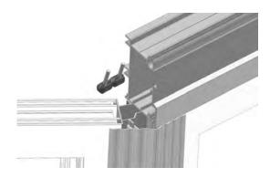
Please note: One double bolt retainer is required per bar however a single bolt retainer (C9144) is required for each starter bar and either side of the eaves beam (A5080) corners for the hip bars. Do not throw any bares away.
