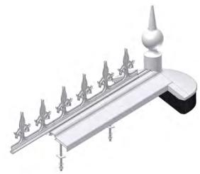
The last piece of cresting may have to be cut to length so that it finishes flush with the end of the ridge top cover.
