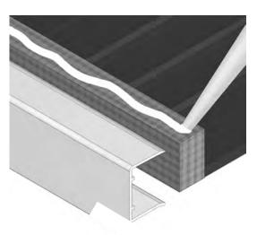
The end closure (P6054) push fits over the bottom edge of the roof glazing sheet with the flange facing down.
