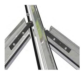
Slide the undercladding back to the top of the jack rafter and tight up against the Georgian hip undercladding, locate the jack rafter onto the bolts in the eaves beam and loosely attach the M5 flange nuts.
