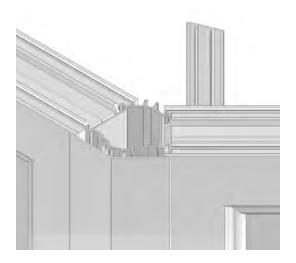
Select the 18mm coupling covers (P111) and position onto the recesses on the sides of each quarter turn button (C105) positioned on the 18mm inline couplings (A104) and press home.
