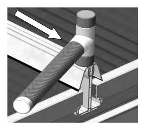
When the bar top cap is attached, make sure that the bottom face of the bar top cap is flush with the bottom face of the bar. Remove the protective film from the bar top cap. Repeat for all top caps.
