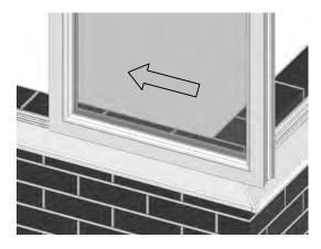
The sill support block (C106) will sit in the 150mm sill (P106) as shown below.
