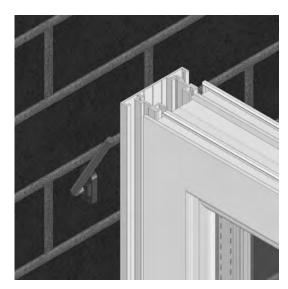
When the quarter turn button (C105) is in position and resting against the two-part connector (A112), turn the 6mm Allen key (6AK) 90° clockwise. The quarter turn button (C105) will 'click' into position.
