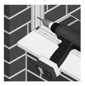
Please note that in dwarf wall models the 26mm wall connector (A105) should be cut to size unless a set of French doors are to be positioned against the wall in which case they are left full height. The French door outer frame is then fitted in the same way as any other panel.
